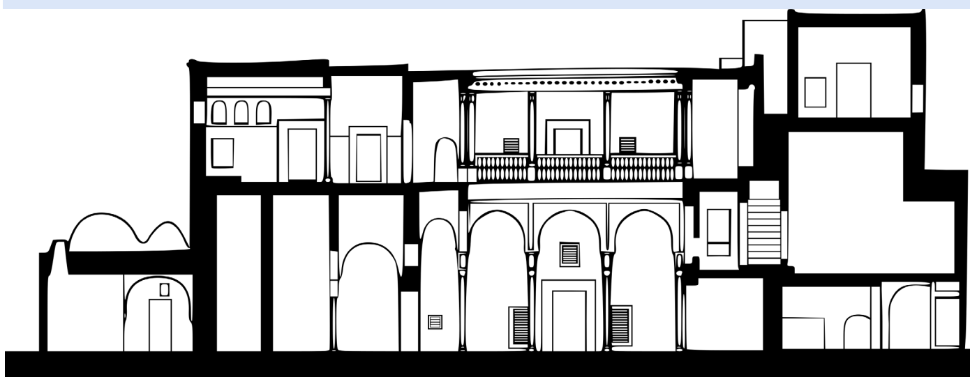
Cross-section of traditional Dar El Haddad courtyard house. © UNESCO / Carlota Marijuan Rodriguez, based on 1967 drawings by the Institut National d'Archeologie et Arts, kept at the UNESCO Archives.
