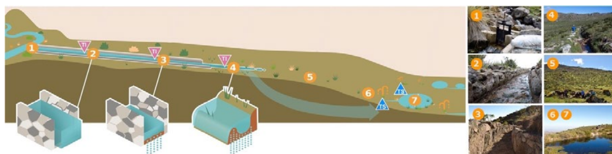
Figure 2. Conceptual representation of the amuna practice. 1. Flow diversion point; 2 & 3: diversion canal; 4. Infiltration in the hillslope; 5. Subsurface flow; 6. Delayed resurfacing of the water.
