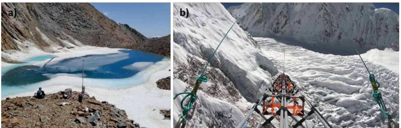
Figure 3. A novel, ‘Big Thaw’ lake sensor set up to monitor snowfall in the Alps. b) The new helicopter radar system surveying glacier ice thickness over the Khumbu Ice Fall in the Western Cwm of Everest, Nepal. (Photos: Pritchard).
